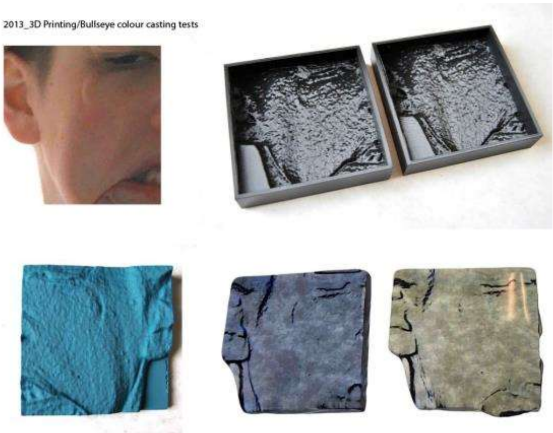
Figure 58 3D printed mould negative for glass casting
