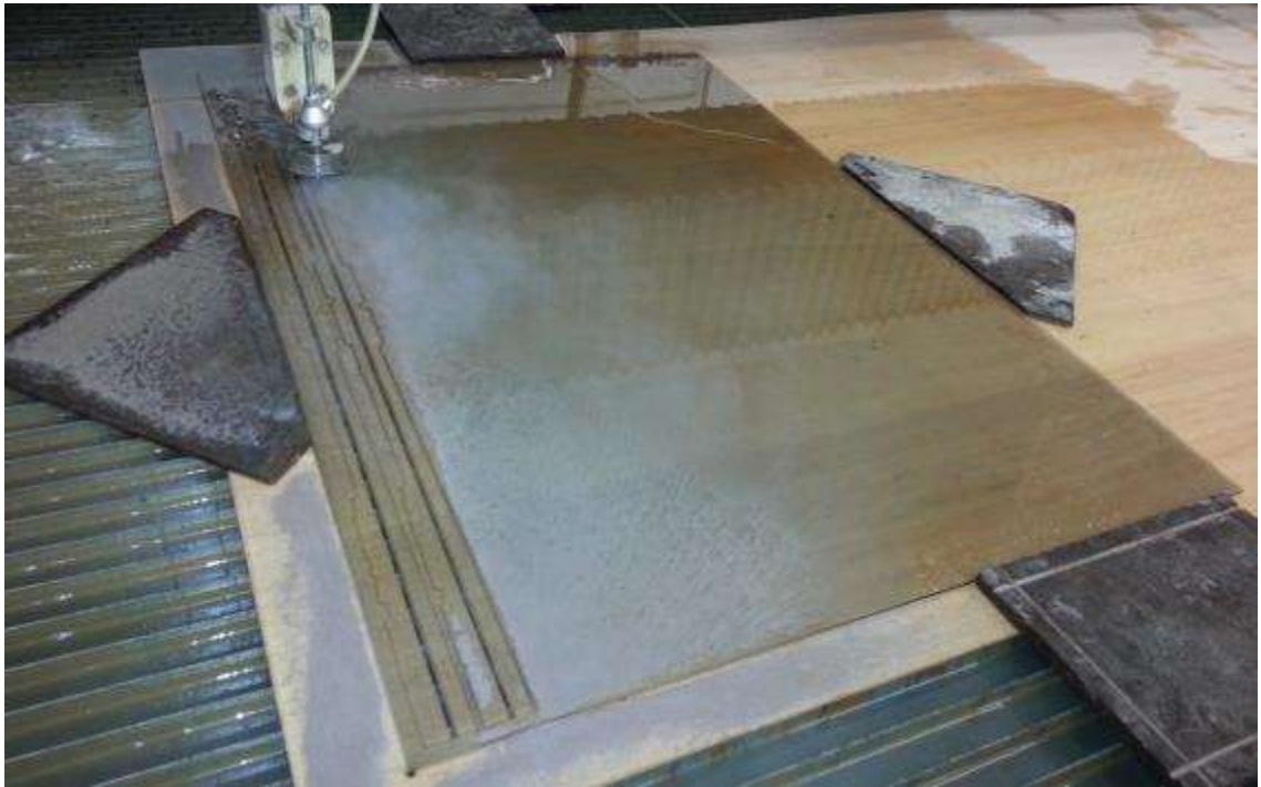
Figure 31 Waterjet cutting contours from float glass sheet
