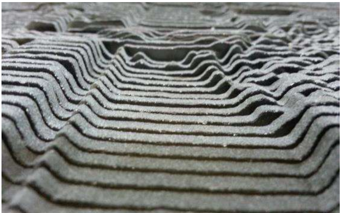
Figure 34 Detail of Window contours prior to kiln-forming
